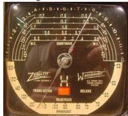
switches. The set was found not to be working on the upper short wave bands (above around 12MHz). A weak local oscillator tube was suspected and so this was replaced with a tested 1LE3 tube from SPARC stocks. This done (and the fault cured), the upper bands were re-aligned and the set was then soak-tested for around 8 hours and found to be working well on all bands. The dial cord was found to be slipping intermittently and a little powdered rosin was rubbed onto it to effect a cure.
