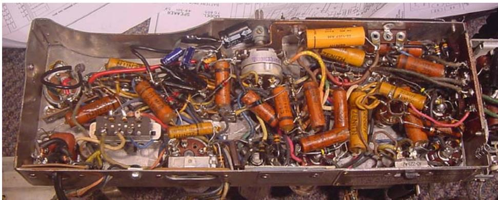
Continuity checks were then made on the tube heater circuits - all seemed in order and, with the speaker connected, power was applied via a Variac. At about
