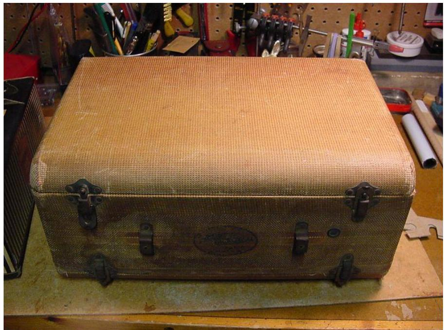
design (mains or battery operation) evolved quickly into the 6G601M 'Sailboat' (6 tube), and by 1942 into the first (7 tube) TransOceanic design, the 7G605 'Clipper' and 'Bomber' styles (all named after the speaker grill designs). These rugged, utilitarian set could receive five shortwave bands (49, 31, 25, 19, and 16 meters) in addition to the regular AM
