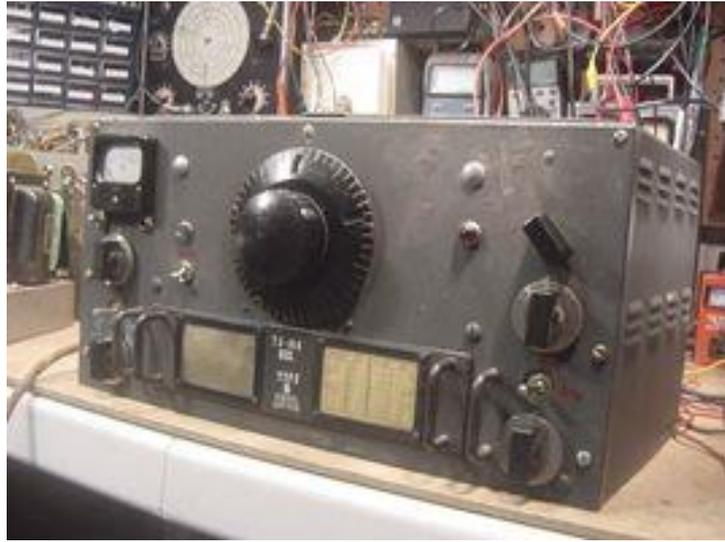
leading to increased stability. The tuning mechanism is built like a tank and the famous ‘PW’ tuning dial is a marvel of engineering. Frequency is read out from a scale on the dial marked 0 to 500, and this vernier reading converted to frequency using a chart supplied with each coil pack. This system facilitated re-setting the set to the same frequency but was of less uses for ‘bandcruising’ use.
