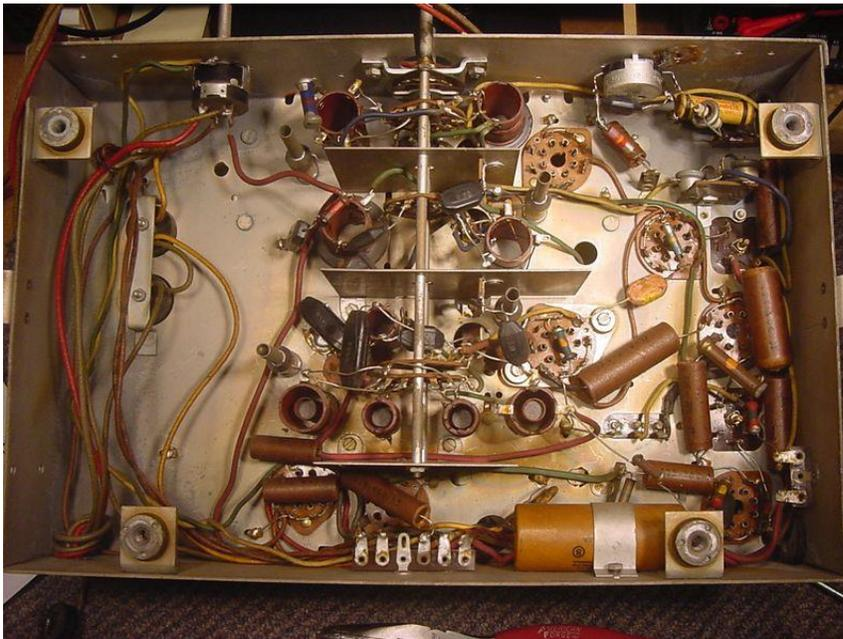
Mechanical work undertaken on the chassis included freeing the tuning mechanism, which was seized completely - using WD40 to free/clean it and then a light application of thin machine oil to the mechanism to keep it running smoothly. This chassis is one of the more complex battery sets, as most cover only the Broadcast Band plus (maybe) one short wave band. By the time this set was manufactured (around 1938) most sizeable
