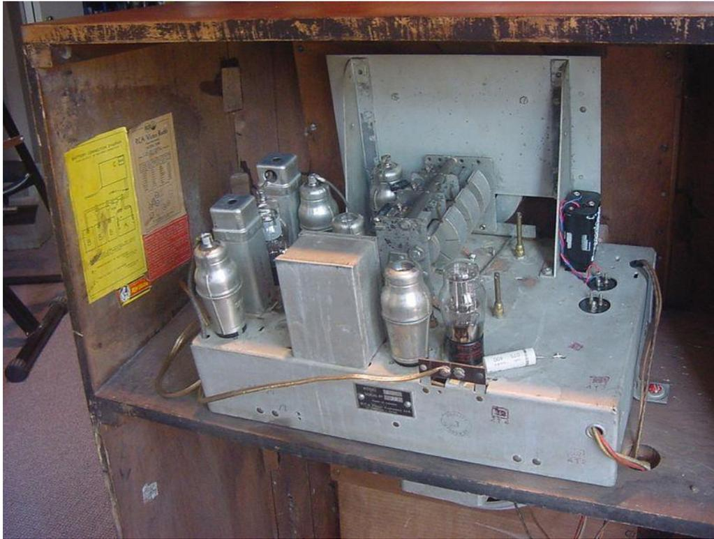
Now, not liking the idea of all those batteries, a neat little mains power supply was designed and built for this radio (and which is suitable for other battery sets). Many power supplies designed for this type of service are designed for smaller radios with 1.5v filaments and a 90 volt plate
