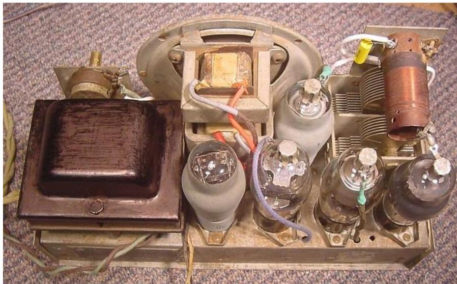
the re-build. The wires emerging from the power transformer are wrapped in what looks like bandages, however, some of this looked suspiciously fibrous, possibly containing asbestos. Not being able to remove this without dismantling the transformer, it was 'stabilized' in-situ by applying several coats of clear nail varnish.
