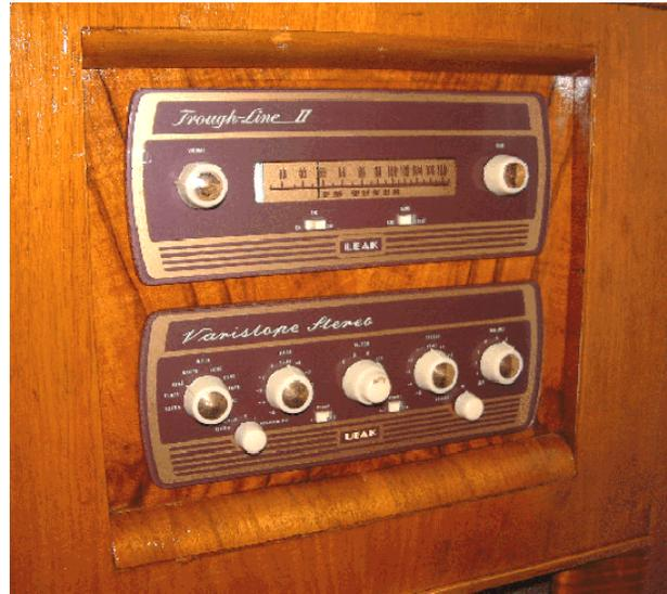
The MkII Trough-Line was originally issued as a mono unit, with provision for adding a stereo de-multiplexer later. Subsequent models were also available with solid-state stereo decoders.
