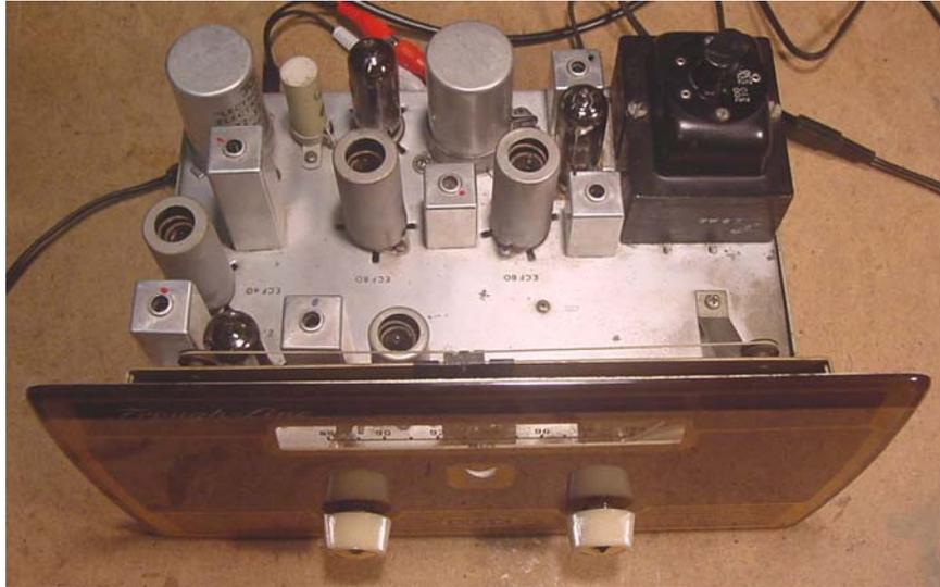
The Leak MkI and MkII tuner's circuit design was rather sophisticated for its day, featuring a cascade RF amplifier and a cathode-follower AF stage, the use of the trough-line tuning element and adjustable quieting ('squelch') to eliminate inter-station noise. In addition, the Mk II incorporated a switchable automatic frequency control (AFC), output for a stereo decoder and used solid-state diodes in the discriminator circuit.
