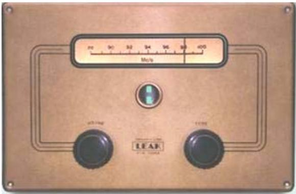
Above: a very early Leak Trough-Line Mk1 FM tuner with the pressed steel front, dating from around 1955.
