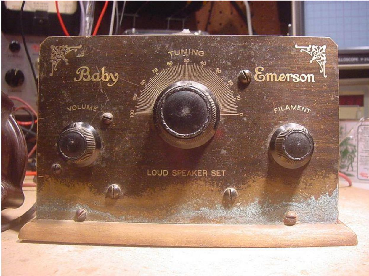
capacity-coupled to the grid (G2) of the third triode, the coil of the horn speaker forming its anode load. Volume control is effected by a grounded series-tuned circuit inductively-coupled to the main tuned circuit coil. The 'Filament' control adjusts the filament voltage via a 20 ohm rheostat. The set requires a 6volt at 0.25A supply for the filaments (adjusted to provide 5v via the rheostat), 45volts for the detector
