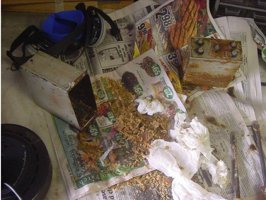
electrolytics (6 x 10uF 450vw units—3 series pairs to give 3x5uF 900vw units as the HT in the radio reaches over 500v when in standby mode). Following this, the radio was cautiously powered-up and it worked first time. A few capacitors were changed (mainly as a precaution) and a recommended minor modification carried out to the AF output stage
