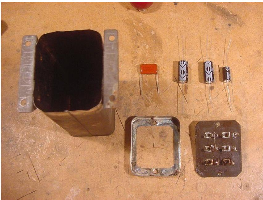
was only touched-up where needed (using a furniture touch-up pen) and then cleaned using lemon oil and polished with wax. However, inspection of the chassis revealed that it had several 'battle scars' where several previous repair attempts had been undertaken, testament to this being a well-used radio over the years. Replaced components included the push-pull driver transformer (replaced with a Thoradsen unit), the smoothing choke (replaced with one so large
