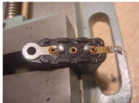
original 'dog bone' carbon resistors checked out of tolerance and so were replaced with modern metal-film types (no attempt was made to disguise these as 'dog bone' types). The volume control was removed and cleaned using De-Oxit. The tuning gang was carefully cleaned and re-lubricated with molybdenum grease and an in-line fuse was fitted into the power transformer primary winding to provide some protection.
