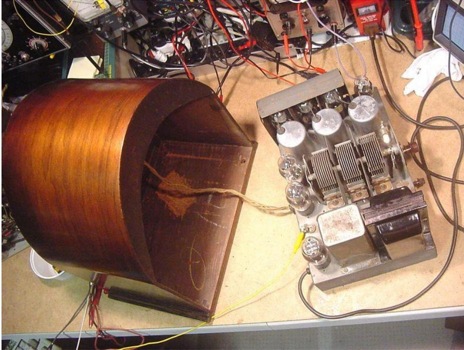
sharp cut-off screen grid tubes in the tuned RF stages, another #24 as a tuned-grid detector, a #27 triode as first the audio amplifier, a pair of #71A triodes in a push-pull output stage and a #80 rectifier in the power supply. A high level of metal screening was used to isolate the RF coils from each other and to screen the RF and detector tubes. The number of passive components is minimal:
