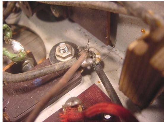
All paper capacitors were replaced (the one across the filter choke was a dead-short and all others were leaky/low capacitance), and new
