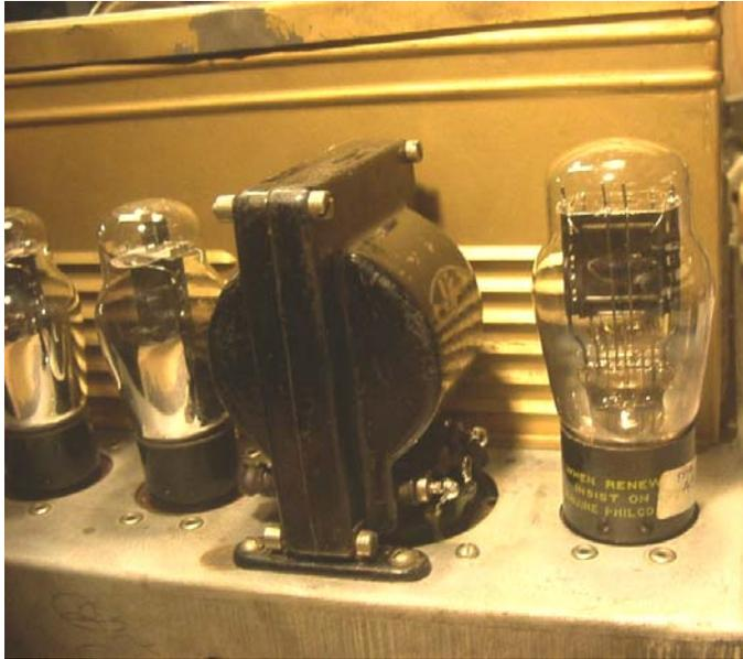
did the RF and audio output transformers, the power supply filter choke and the loudspeaker field coil. However, the audio driver transformer primary was found to be open-circuit. A suitable part was sourced from the SPARC museum stock (a late-1920's Ferranti unit) and this was fitted – a bonus of using a 'period' part was that it did not look out of place on the chassis (photo, left).
