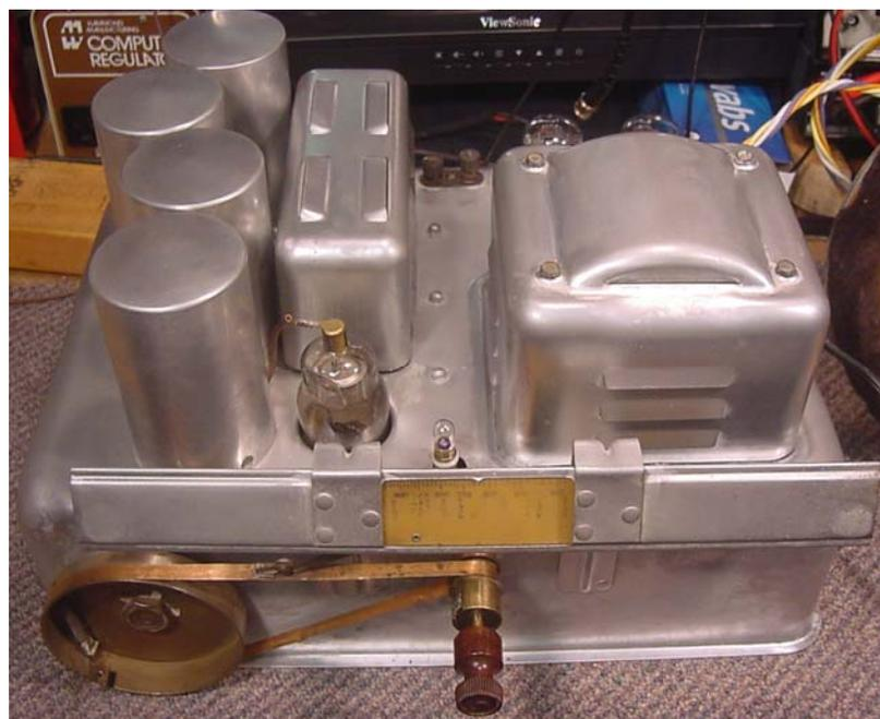
'slide rule' type (one of the earliest I have seen), driven by an actuating rod linked to the top of a pair of very robust brass bands coupled to a large wheel on the tuning gang. Another nice touch on this chassis is 'Brunswick' moulded into the each of the tuning gang rotor plate castings
