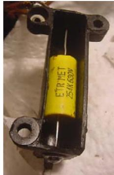
of the Bakelite-cased capacitors were replaced (all were leaky), five of the cases were re-stuffed (photos, left), however, the two more inaccessible ones were not re-stuffed, but instead the replacements were placed discretely in the wiring. Two of the capacitors in the large can
